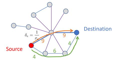
Link duty cycle estimated by an L-layer graph convolutional neural network (GCNN)
